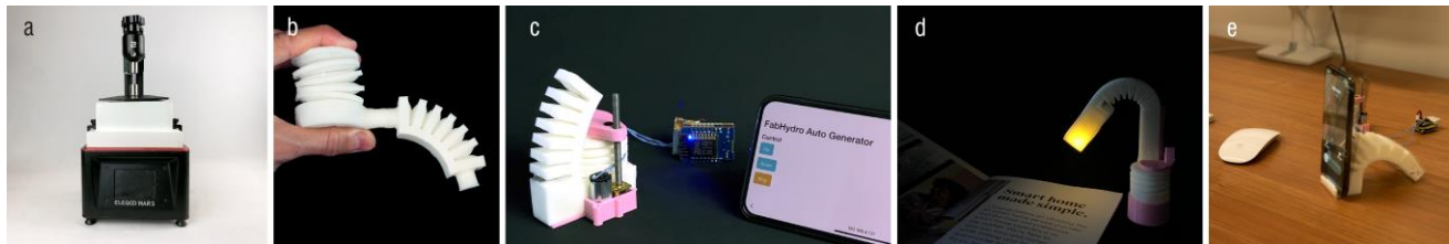
Figure 1 – FabHydro : a) an off-the-shelf SLA printer with a modified tank and printing plate; b) a complete hydraulic device produced by FabHydro ; c) a bending actuator is activated by an automatic generator; d) a printed lamp lights up with the change of its posture; e) a phone stand acts as an ambient display when the phone rings.
